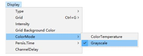
There are two kinds of grayscale display mode, When choosing a DPO mode for level 256 grayscale display and the max waveform capture rate to 60,000 wfm/s, but if the Acquire is on the FastAcq model,so the oscilloscope is only with 1-level intensity grading display function and the max waveform capture rate to 400,000wfm/s.
