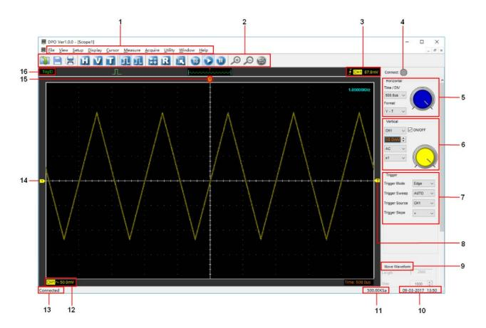
In addition to displaying waveforms, the display area is filled with many details about the waveform and the oscilloscope control settings.
