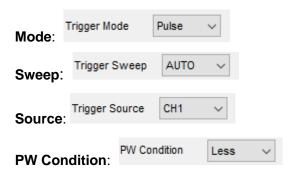
**Pulse Width**: The Pulse Width adjust range is 10ns~10s. When the condition is met, it will trigger and acquire the waveform.
