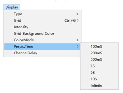
With persistence, the oscilloscope updates the display with new acquisitions, but does not immediately erase the results of previous acquisitions. All previous acquisitions are displayed with reduced intensity. New acquisitions are shown
