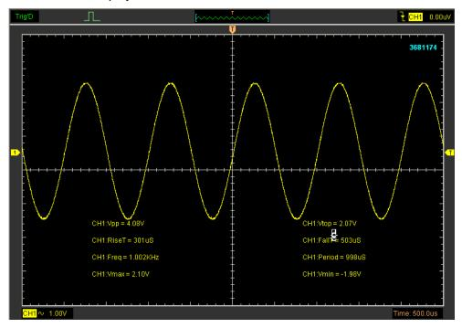
**Note**: The results of the automatic measurements will be displayed on the bottom of the screen. Maximum 8 results could be displayed at the same time. When there is no room, the next new measurement result will make the previous results moving left, out of screen.
