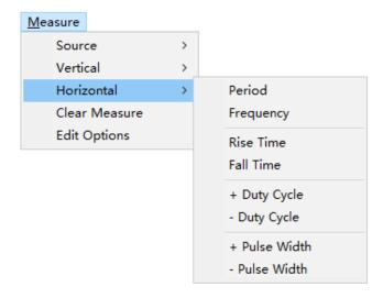
**Period**: Time to take for the first signal cycle to complete in the waveform
