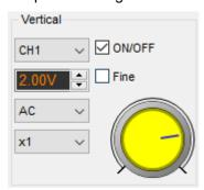
**Note**: The attenuation factor changes the vertical scale of the oscilloscope so that the measurement results refect the actual voltage levels at the probe tip.
