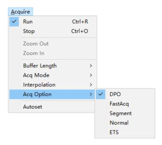
**DPO:** In this mode, the oscilloscope supports 256-level intensity grading display with one channel. The Max Waveform capture rate up to 60,000 wfm/s.
