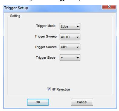
The user can turn on "HF Rejection" to eliminate trigger higher-frequency (20M above)
