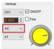
You can set the coupling to **DC**, **AC** or **GND**. If you set the coupling to **DC**, it blocks the **AC** component of the input signal.
