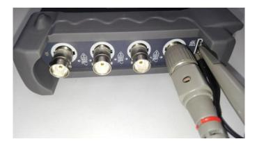
2. Set the CH1 probe attenuation of the oscilloscope to X10. (The default is X1).
