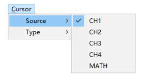
The user can set the source to **CH1**, **CH2**, **CH3**, **CH4** and **MATH**. When you use cursors, be sure to set the **Source** to the waveform on the display that you want to measure.
