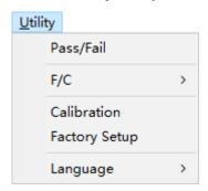
When you click the **Factory Setup** in **Utility** menu, the oscilloscope displays the CH1 waveforms and removes all other waveforms.
