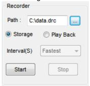
This function can record input waveform form CH1, CH2, CH3, CH4.
