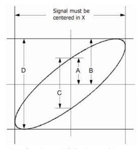
$Sin\theta = A/B \text{ or } C/D$ , where  $\theta = phase shift (in degrees) between the two signals.$
