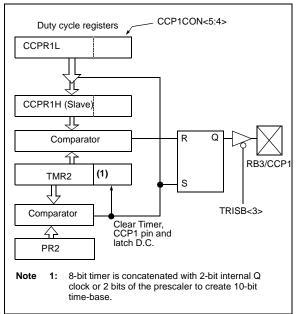
A PWM output (Figure 9-4) has a time base (period) and a time that the output stays high (duty cycle). The frequency of the PWM is the inverse of the period (frequency = 1/period).
