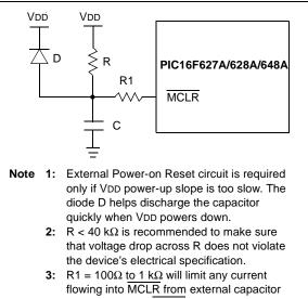
flowing into MCLR from external capacitor C in the event of MCLR/VPP pin breakdown due to Electrostatic Discharge (ESD) or Electrical Overstress (EOS).
