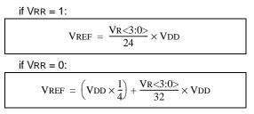
The setting time of the Voltage Reference must be considered when changing the VREF output (Table 17-3). Example 11-1 demonstrates how Voltage Reference is configured for an output voltage of 1.25V with VDD = 5.0V.
