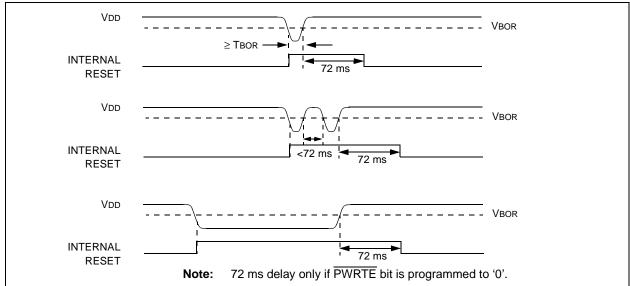
FIGURE 14-7: BROWN-OUT SITUATIONS WITH PWRT ENABLED
